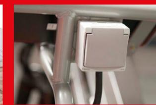
**230 V European type electric plug with differential circuit breaker**
