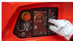
The large screen at the lower control box offers additional information to the top control box for operator and allows technicians to carry out a quick diagnosis, consult the machine memory and many
