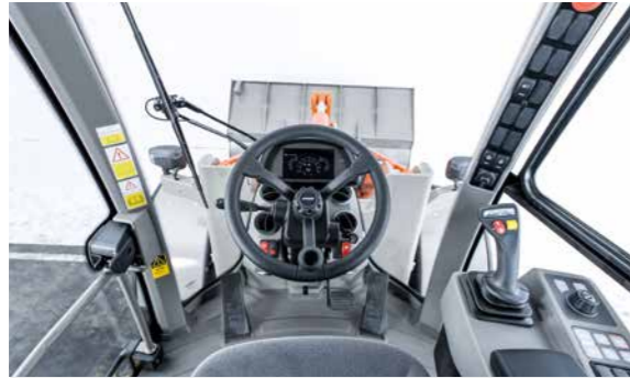
Front: Unobstructed view at floor level without steering column blockage
