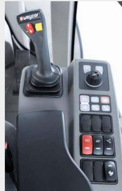
Control & operating elements: Reduced elements for intuitive operation, joystick moves ergonomically with the seat and fits any hand size
